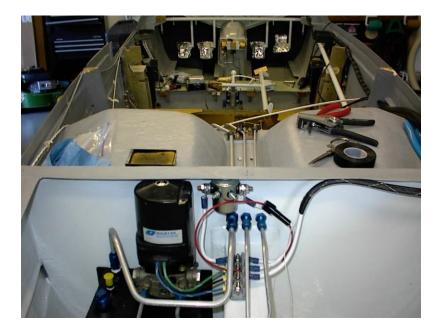
An accumulator acts as a "shock absorber" in the system. A check of flap operation with the system "off" will tell you if the accumulator is working – you should be able to cycle the flaps up and down with pump off.
