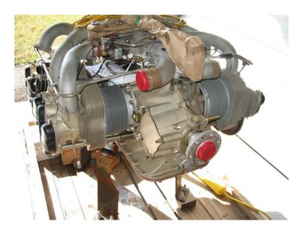
At takeoff power of 2700 rpm and 38(A,B) or 38.5 (E) in. Hg., the TSIO-550 develops 350 horsepower. The engine may be operated at maximum takeoff power in the climb to cruise altitude. Maximum recommended cruise power setting is 2500 rpm and 31.5 in. Hg., which yields 263 horsepower or 75% power. The engine is equipped with two Airesearch turbochargers and dual intercoolers. Overboost protection is provided by a pressure relief valve to limit compressor discharge
