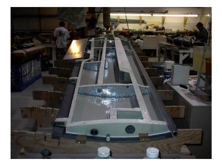
The aircraft has two wet wing fuel tanks. The fuel tanks vary in size from 80 gallons to 110 gallons and run from the inboard to outboard end of each wing. The tanks are vented to the outside atmosphere by ports on the bottom of the wingtip and each cell has flush type filler caps mounted above the cell. There are one or two low point drains on each wing. Fuel runs into a baffle tank on the inboard end of
