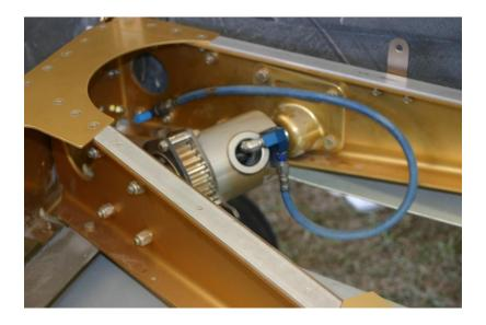
The mains and the nose gear are held up by hydraulic pressure. The mains have mechanical down locks in the hydraulic actuating cylinder and a 110 psi gas shock strut provides a positive down/lock for the nose gear. There is no "uplock " on the mains. During condition inspection check operation of the mechanical downlock.
