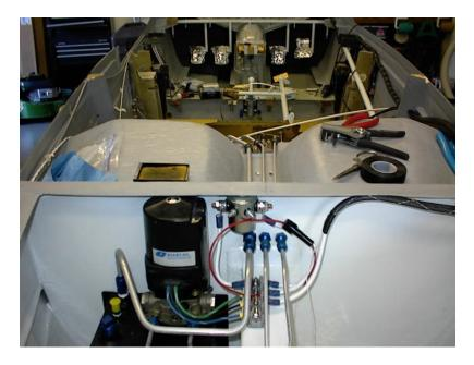
An airspeed switch mounted on the pitot tube line prevents gear retraction below 75 kts. For landing gear retract tests on jacks you must blow into the pitot tube to get enough "airspeed" to disengage the airspeed safety switch. A balloon will also do the trick. The main gear is retracted into the fuselage via full rack and pinion gears, and the nose gear also retracts aft.
