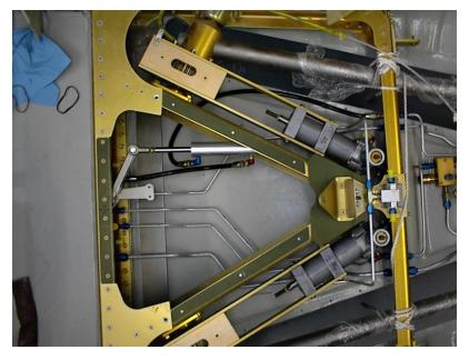
The flaps are operated by a flap valve mounted below the throttle quadrant and are selectable to any setting between zero and forty degrees. Electrically or
