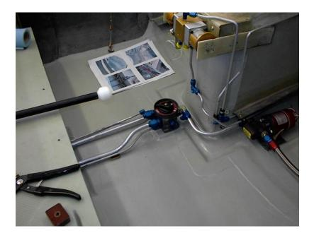
Fuel flows from the selector value to an electric boost pump located on the floor or sidewall and then through the firewall to the fuel filter/ sump. The boost pump has an overboard drain should the pump diaphragm fail.
