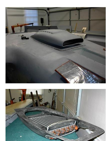
The evaporator is mounted in the aft cabin and supplies chilled air to the cabin. It is controlled by a switch on the instrument panel.
