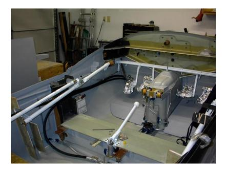
All primary flight controls use centerline hinging on bearings. The ailerons and
