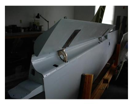
The hydraulically driven fowler flaps extend from aileron to fuselage on each wing.
