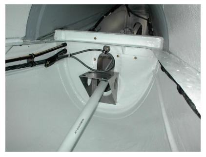
elevator is push rod actuated. Both side stick controls have positive grip handles and should have a radio transmit button mounted on them. Other switches may be mounted on the grips. The rudder pedals actuate the rudder with stainless
