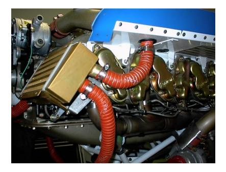
This air is also routed to the mixing valve. It is close to ambient air temperature. A cockpit control cable selects temperature from a mix of these two air supplies. Additionally, another control cable selects an overboard dump of all engine air for unpressurized flight, or for smoke in the induction system. The flow of compressed air into the cabin is regulated by an outflow valve that keeps the pressure constant by releasing excess pressure into the atmosphere.
