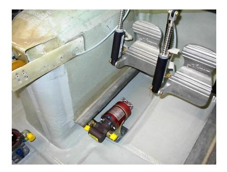
The sump should be drained often to keep water and debris out of the engine. Annually, it should be disassembled, cleaned and reassembled per the Lancair drawings.
